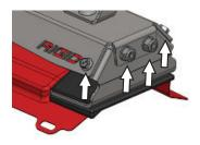
Install the corner M6X1.0 bolts with a 10mm socket loosely with blue thread locker. Once all corner bolts are installed, tighten 4 side carriage bolts and the corner bolts.
