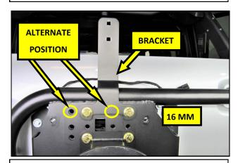
**44.** Mount the Lower Brake Light Bracket to the Tire Carrier using two Large Flange Bolts. Torque the Bolts to 45 lb.ft. **NOTE:** The Lower Bracket can be mounted off center, towards the drivers side to be more centered with larger tires. There is also sufficient bolt length for the Hub flange and the Light Bracket to use the same holes.
