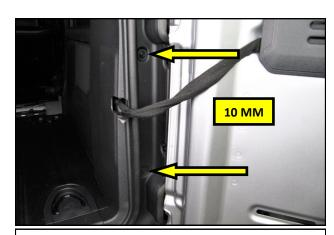
**14.** Using a 10 mm socket, remove the two screws in the hinge cover.
