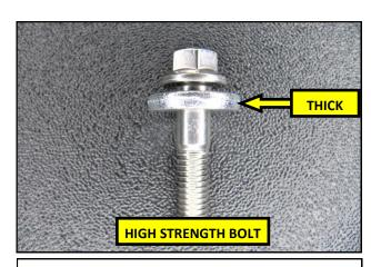
**20.** The High Strength, ARP® bolts and Thick Washers are to be used for mounting the Inner hinge to the vehicle. **NOTE:** The RTR Upper and Lower Hinges have location specific profiles. Match The RTR Inner Hinge to the marking in step **17** before installing the Hinge.
