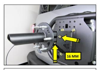
**37.** Feed the Extension Harness through the Hub and slide the Hub into the Base as shown. Thread two of the M12 Flange Nuts into the Adjuster Bracket. Leave the Bolts snug for now.
