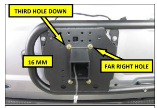
**35.** Feed the Camera Extension Harness in through the bottom of the Carrier Base. Mount the Carrier Base as shown, using the M12 (large) Flange Bolts and torque the Bolts to 45 lb.ft. The recommended mounting position is intended to accommodate up to a 35" tire with the stock bumper. The Base can be moved to accommodate larger size tires and RTR Accessory Plate options.
