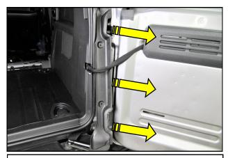
**15.** Remove the hinge cover from the vehicle and set it aside.
