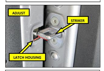
**26.** To compensate for added weight of the spare tire, RTR suggests adjusting the tailgate upward until the latch housing is in slight contact with the striker. The actual amount of upward adjustment will vary depending on tire size & weight.
