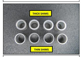
**INSTALL OPTION A.** RTR has included two sets of Position Control Shims—Thick and Thin. With additional weight of larger tires, Fuel cans, or trail jacks added to the Tire Carrier it may be necessary to readjust the tailgate position to compensate.
