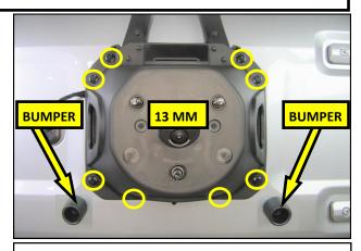
**2.** Using a plastic trim removal tool, pry the rubber bumpers out of the tailgate. Remove the eight bolts securing the OEM tire carrier to the vehicle and set them aside.
