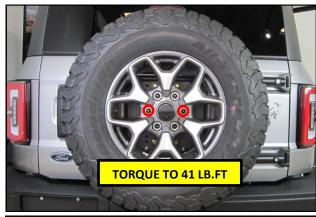
**54.** Install the 2 remaining Lug Nuts and torque all six to 41 lb.ft.
