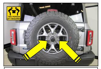
**51.** With the help of an assistant, slide the spare tire onto the RTR Tire Carrier. Take caution to avoid cosmetic damage to the powder coat finish.
