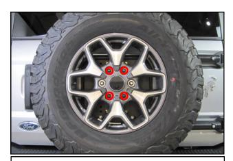
**52.** Using four of the supplied Spline Drive Lug Nuts and Socket, snug the spare tire down onto the RTR Tire Carriers Hub.
