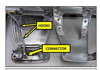
**10.** Separate the two halves of the housing to gain access to the light. Unhook and disconnect the wiring harness.
