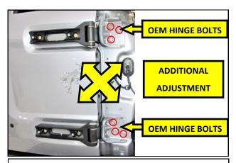
**INSTALL OPTION B.** Because of varying manufacturing tolerances and or severe off roading, additional tailgate adjustment may be needed and can be found behind the right tail lamp. loosen the six OEM hinge bolts and align the tailgate as needed. Torque the bolts to 30 lb.ft.
