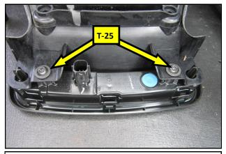
**11.** Using a T-25 TORX® driver, remove the two screws in the brake light bracket and remove the bracket.
