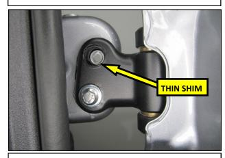
**A2.** These Shims can be inserted, one at a time, into the Inner Hinge Flanges to help control movement. Any combination of Thick and Thin Shims can be used. Any unused Shims should be retained for possible future use.
