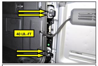
**49.** Torque the 4 Inner Hinge Bolts, final tight to 40 lb.ft.
