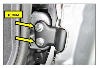
**23.** Using the High Strength Bolts and Thick Washers, mount the Lower Hinge onto the vehicle as shown. Leave the bolts snug at this time to allow for final adjustment.
