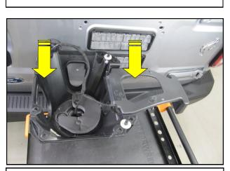
**3.** Set the tire carrier onto a tool cart or equivalent.
