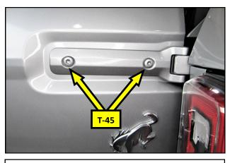
**19.** Using a T-45 TORX® driver, remove the two upper exterior hinge bolts and set the hinge aside. The OEM hinge and hardware will not be reused in this installation.
