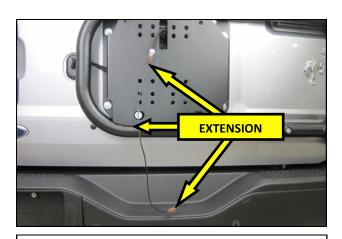
**34.** Select the appropriate Camera Extension Harness (Coaxial or 6 Pin) for the application and connect it to the OEM harness as shown. Discard the unused Harness Extension. It will not be used.
