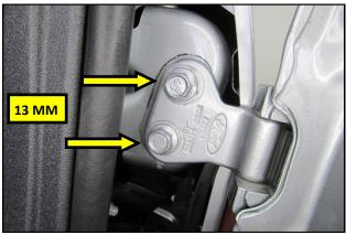
**18.** Using a 13 mm socket, remove the two upper, interior hinge bolts.
