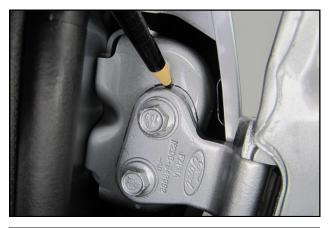
**17.** Using a grease pencil or equivalent, mark the position of the upper and lower tailgate hinges onto the vehicle as shown.
