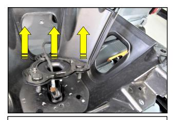
**7.** Remove the steel bracket and camera assembly from the tire carrier.
