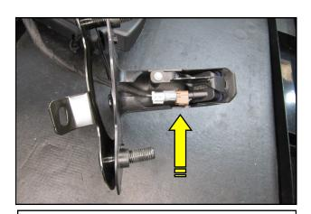
**8.** Disconnect the camera harness from the camera assembly and set it aside.
