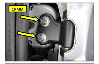
**21.** Using the High Strength Bolts and Thick Washers, mount the Upper Hinge onto the vehicle as shown. Leave the Bolts snug at this time to allow for final adjustment.
