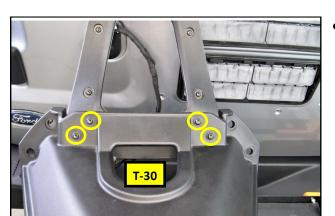
**5.** Using a T-30 TORX® driver, remove the four screws securing the third brake light to the tire carrier.
