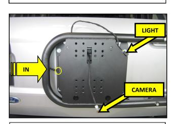
**33.** Feed the camera and brake light harnesses through the opening on the side of the Carrier. Feed the camera harness out through the front of the Carrier and the brake light harness out through the top as shown.
