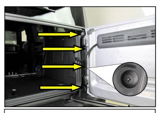
**13.** Open the tailgate to expose the hinge cover. Using a No. 2 Phillips driver, remove the four plastic rivets in the cover
