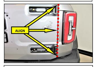
**25.** Carefully close the tailgate. Check the tailgate to body alignment and adjust as necessary, leaving all hardware snug at this time to allow for final adjustment.
