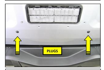
**28.** Insert the supplied Low Profile Plugs into the tailgate bumper holes in the from step 2.
