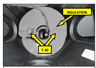
**4.** Using a T-30 TORX® driver, remove the two plastic fasteners in the insulation pad and remove the insulation from the tire carrier.
