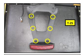
**9.** Using a T-25 TORX® driver, remove the six screws in the third brake light housing.
