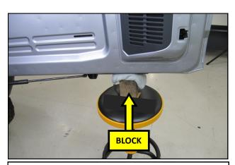
**16.** Using a shop stool and a padded block of wood, support the bottom of the tailgate as shown.
