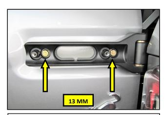
**22.** Install the RTR Upper Hinge onto the tailgate as shown, using the supplied M8 Flange Bolts. Leave the Bolts snug at this time to allow for final adjustment.
