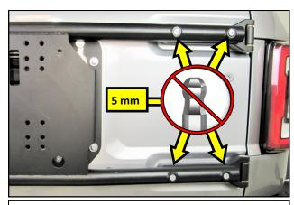
32. Using a 5 mm hex bit socket, in like new condition, carefully install the Flat Head Bolts through the Hoop arms and into the RTR Hinges. Do not use a ball driver bit for this step. Torque the flat head Bolts to 17 lb.ft. Torque the remaining Tire Carrier Bolts from Steps 29, 30 and, 31 to 30 lb.ft.
