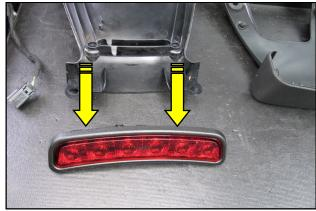
**12.** Remove the brake light from the housing and set it aside, This light will be reused with the RTR tire Carrier.
