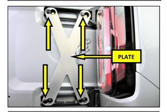
**27.** Using four of the OEM tire carrier bolts from step **2**, mount the Alignment Plate to the Upper and Lower Hinges. Once proper positioning has been achieved, torque all four exterior Hinge Bolts final tight-30 lb.ft. Remove the OEM bolts and Alignment Plate. RTR Recommends retaining the Alignment Plate for future use.
