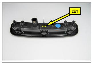
**41.** Using a pair of diagonal cutting pliers, carefully trim off the center post on the back of the OEM brake light.
