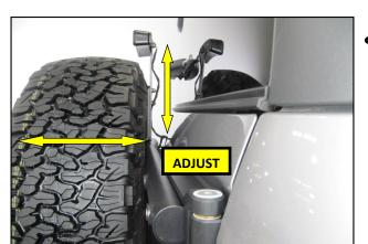
**53.** Check tire to Carrier clearance and adjust if necessary using the two bolts from step **37**. Once the proper position is achieved, torque the Bolts to 45 lb.ft Adjust the brake light height if necessary using the Nuts from step **44**.
