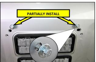
29. Partially install two of the supplied M8 Hex Head Bolts with the Over Size Washers into the top 2 holes in the tailgate.
