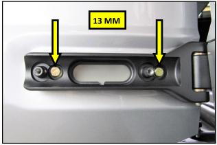
**24.** Install the RTR Lower Hinge onto the tailgate as shown, using the supplied M8 Flange Bolts. Leave the Bolts snug at this time to allow for final adjustment.
