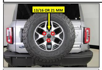
1. With the vehicle parked on level ground, open the tailgate appx. 5 to 10 degrees and remove the spare tire. Note the movement in the tailgate due to the spare tire removal. The noted movement due to tire weight should be accounted for during final alignment.
