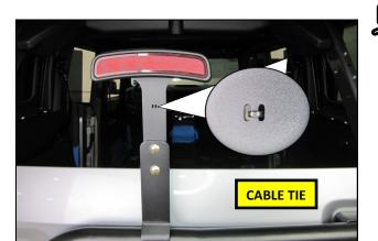
**47.** Secure the wire harness to the Upper Brake Light Bracket using the supplied Cable Tie. Trim the excess length.
