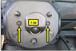
**6.** Using a T-30 TORX® driver, remove the two screws on the face of the tire carrier.
