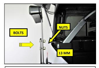
**45.** Join the two Brake Light Brackets together using the two Carriage Bolts and Lock Nuts. The Upper Bracket is slotted and will accommodate larger tire sizes. Torque the Lock Nuts to 14 lb.ft. Threadlocker will not be needed for this step.
