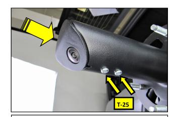
**40.** Carefully Insert the Camera and Mount assembly into the snout on the Hub and secure it using the 2 remaining #10 Pan Head Screws.
