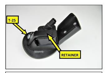
**38.** Transfer the OEM camera into the RTR Camera Mount and secure it using supplied Retainer and one of the # 10 (Large) Pan Head Screws.
