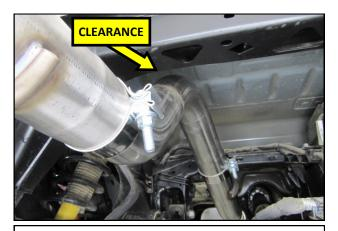
**18.** Adjust the Exhaust into its final position and where the most clearance can be gained under the crossmember. Tighten all 4 of the exhaust Clamps to 45 lb.ft.
