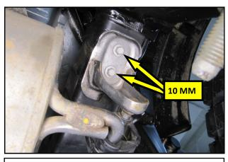
**7.** Using a 10 mm socket, remove the two bolts securing the driver side muffler hanger to the frame. With the help of an assistant, remove the muffler and hanger from the vehicle.
