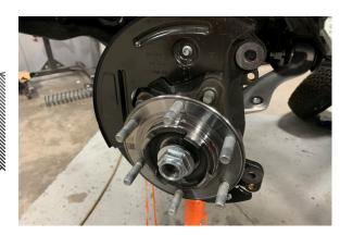
17. Break loose but do not remove the upper and lower ball joint 18mm nuts. Use a ball joint separator tool to detach the ball joints from the spindle. Alternatively with a hammer, you can strike the ball joint boss on the spindle to remove the ball joint.
