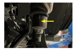
18. It is important to be careful, as the control arms may be under tension. Once free, support the spindle as you remove the upper and lower ball joint nuts. Allow the spindle to droop as you slide the axle shaft out of the hub.
