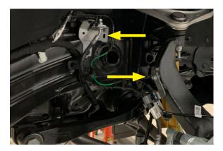
14. Remove the 18mm brake caliper bolts and hang the caliper securely in the wheel well to prevent from overstretching the brake hoses.
