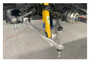
19. Remove the 18mm bolts fastening the hub to the OEM spindle. Detach the hub and backing plate then mount them onto the new Belltech spindle using the original hardware. Torque the four bolts to 129 ft lbs.
