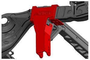
61. Insert the supplied M16 bolt, from front to back through the new bracket and the original frame side track bar hole. Ensure the steel crush tube is on the bolt side and only use a washer on the nut side. The nut should be on the back side of the bracket facing the rear of the vehicle. Fasten but do not torque yet.
