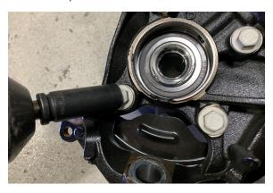
20. Remove the three 15mm top mount nuts holding the strut to the chassis and the two lower strut 18mm nuts. Lower the control arm assembly to gain clearance for the strut to be removed from the vehicle.
