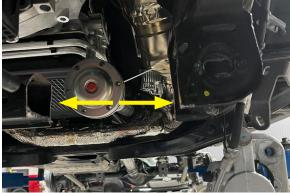
33. To add clearance on the differential, use a grinder to remove the small lobe near the rear upper mounting holes (reference the images below).
