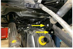
74. Remove the protective covers on passenger control arm bolts.
