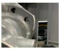
34. If the front differential has the large coupler on the passenger side, you must cut off or grind the small aluminum protrusion on the back side of your power steering rack as shown (reference the images below).
