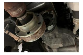
27. Securely support the front differential with a jack, then remove the passenger side differential support 13mm bolt two and the two 18mm bolts on the back of the differential above the input shaft.
