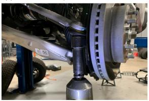
12. 11. Using a 8mm socket, detach the wheel speed sensor from the spindle. Secure the wire assembly away from the working space.
