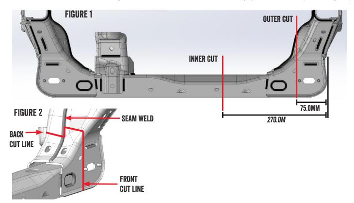
31. On the back side of the rear cross member, measure 7mm inward from the inner alignment pin and mark a vertical line, then wrap the paint pen line up and around to the seam weld. The two lines will be offset and not meet. Connect the two lines along the seam weld.
