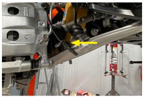
13. Using a 10mm wrench, detach the front ABS and brake line bracket from the spindle and remove the bracket from the chassis.
