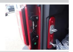
Locate the taillight housing and separate the connectors, taking care not to damage the locking tabs. Repeat this on the other side of the vehicle.
