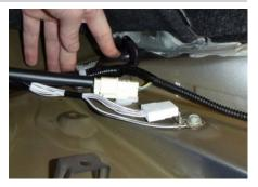
Route the 4-flat along the top of the driver-side frame rail to just behind the driver-side front tire. Loosely secure any excess wire so that it is not drooping or dangling and tighten later.
