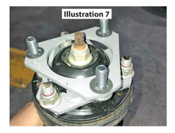
[Illustration 7] Insert 3/8" X 1-1/4" carriage bolts into the top of the strut spacer (55-01-9720). Slide push nuts onto the carriage bolts to hold bolts in place for installation.
