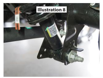
**STRUT ASSEMBLY** [Illustration 8] Remove the lower strut mount hardware. [24mm]
