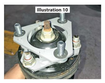
Attach the strut spacer assembly onto the top of the strut by aligning the strut spacer assembly onto the three (3) factory studs. Secure using the factory hardware. [15mm] (40)
