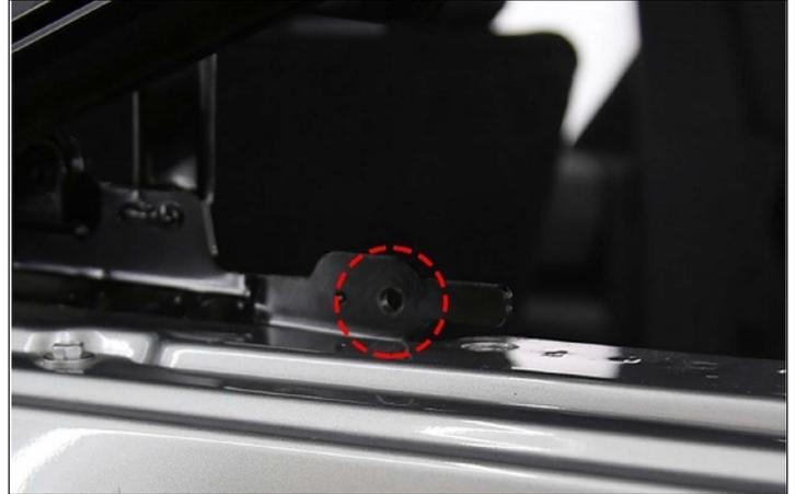
2. Install the supplied long ball stud and washers. Ensure the ball is pointing to the inside of the vehicle. Tighten hardware. Repeat on the other side.
