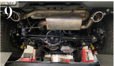
WARNING: Use extreme caution during installation. Torque all fasteners according to manufacturer's torque values and tightening sequence. DO NOT use air impact tools to tighten fasteners on Borla Performance Exhaust Systems. Use of such tools may result in bent flanges or gasket contact areas leading to exhaust leaks.
