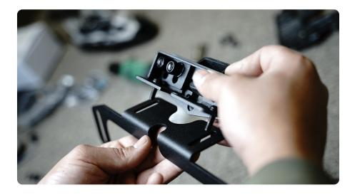
STEP 16 | Align the camera assembly and brackets so that the camera is sitting straight and even on the bracket.
