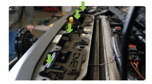
STEP 6 | To remove the grille, pull carefully on the grille towards the front of the vehicle to un-fasten the clips securing the grille. Start at the sides and work towards the middle.
