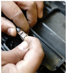
STEP 8 | Use a trim clip tool to remove the clips securing the camera hose to the grille and place it off to the side.
