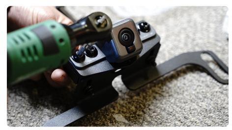
STEP 17 | Install the included extended camera wire to the camera (blue connector) and the press on the included hose onto the factory washer nozzle barb.
