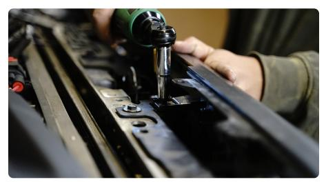
STEP 26 | Place the plastic grille trim back into place above the grille and pull the factory air intake cowl. Secure using the factory plastic grille trim using the factory push clips.
