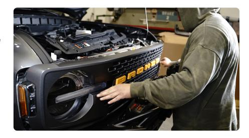
STEP 25 | Use a 13mm socket and the factory hardware to secure the grille to the vehicle.
