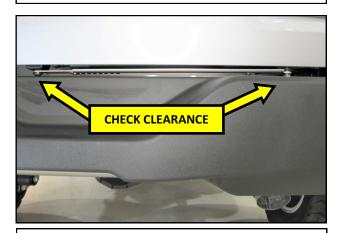
**21.** Carefully close the gate and check for any clearance issues that may be the result of manufacturing tolerances or off road impact. If additional clearance is needed, use the supplied Bumper Shims to space the bumper.
