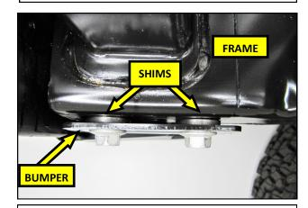
**22.** Remove the lower bumper bolts, one by one, and slide the shims in between the bumper and the frame. With all 4 Shims in place, torque the bumper bolts to 59 Lb.—ft.
