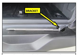
**13.** Set the Bracket and Link assembly onto the rear bumper as shown, with the Ball Stud pointing upward.
