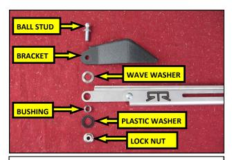
**11.** Create the RTR Body Bracket and Slide Link assembly using the components in the order of the photo above.
