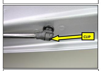
**3.** Using a pocket screwdriver, or equivalent, pry up on the second strut clip to release the strut from the ball stud on the swing gate and set the strut aside.
