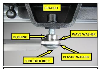
**15.** Create the RTR Gate Bracket and Slide Link assembly using the components in the order of the photo above.
