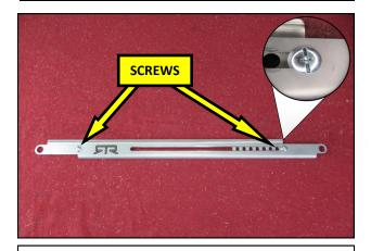
**10.** Create the Slide Link assembly using the two, small Button Head Screws. Tighten the Screws until the threads in the Barrel Nuts end and they stop turning. This will ensure proper thread engagement and allow for movement.
