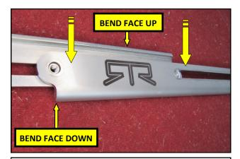
**9.** Align the Upper Slide link with the Barrel nuts and place it onto the Lower link and as shown, with the RTR logo facing up.
