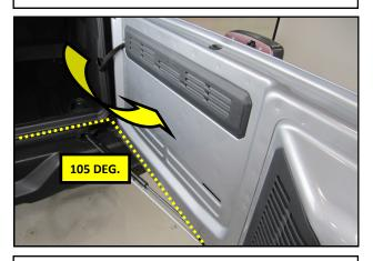
**19.** Open the swing gate until it stops against the Link. Using the adjustment in step **8**, the gate will open approximately 105 deg. and will accommodate most spare tires.
