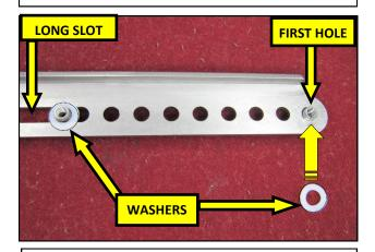
**8.** Place one Barrel Nut into the long slot in the Lower Slide Link and a second Barrel Nut into the first hole at the end of the Link. Place the two Small Plastic Washers onto the Barrel Nuts .
