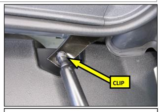
**2.** Using a pocket screwdriver, or equivalent, pry up on the strut clip to release the strut from the ball stud on the OEM bumper bracket.
