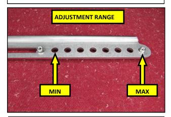
**20.** For vehicles with very large tires, different offsets, or additional gate accessories, the opening can be reduced to prevent a collision with the body or tail light. The adjustment range of the Gate Stop is 80-105 Deg.
