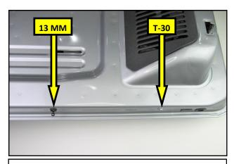
**5.** Using a 13 mm socket and a T-30 TORX® driver, remove the ball stud and the pan head screw at the bottom of the swing gate.
