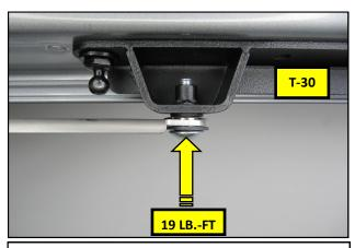
**16.** With the assembly created, and ensuring that the Wave Washer is properly centered on the Bushing, use 40 TORX® driver to torque the assembly to 19 Lb.-ft.
