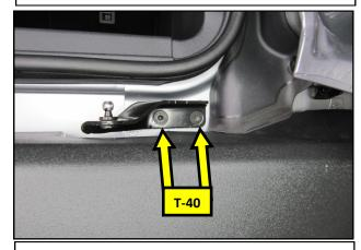
**4.** Using a T-40 TORX® driver, remove the two bolts fastening the OEM strut bracket to the vehicle. Remove the bracket and set it aside.
