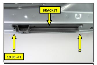
**6.** Mount the RTR Gate Bracket to the swing gate as shown, using the hardware removed in step **5**. Torque the ball stud to 19 Lb.-Ft. Tighten the screw by hand and do not overtighten.
