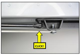
**18.** Install the OEM gate strut onto the ball stud on the RTR Gate Bracket assembly. Verify that the strut clips have fully engaged for proper retention—adjust the clips if necessary.
