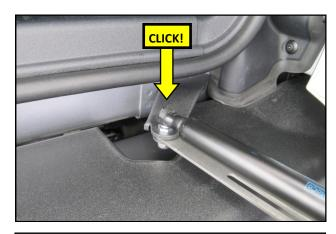
**17.** Install the OEM gate strut onto the RTR Body Bracket Ball Stud. **NOTE:** The strut body (large diameter) is to be installed on the body side.
