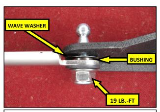
**12.** With the assembly created, and ensuring that the Wave Washer is properly centered on the Bushing, use a 1/2" wrench and socket, torque the assembly to 19 Lb.-ft.
