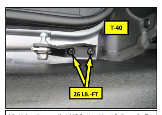
**14.** Using the supplied M8 Button Head Bolts and a T-40 TORX® driver, install the Bracket onto the vehicle. Torque the Bolts to 26 Lb.-ft.
